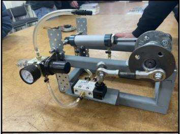
Matthew has made a pneumatic engine that he made for a school project using parts that he sourced from Ebay. He discovered a problem where the flange was not aligned, as the thread was made to imperial standards and the rod was made to metric standard. With some help from Mike Banks, he fixed the rod and got it working at 8psi, though it's rated for up to 100 psi!
