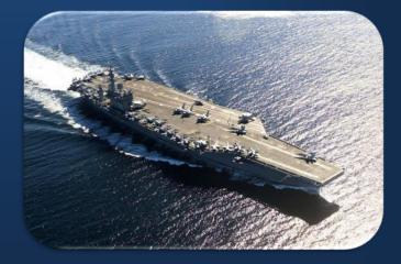
USS Nimitz (CVN-68) - A USS Nimitz class aircraft super carrier. It is 333m long, has two nuclear reactors aboard with a maximum speed of over 30 knots (56 hm/h) along with an unlimited range over 20 years.
