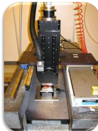
A device designed to facet diamonds
