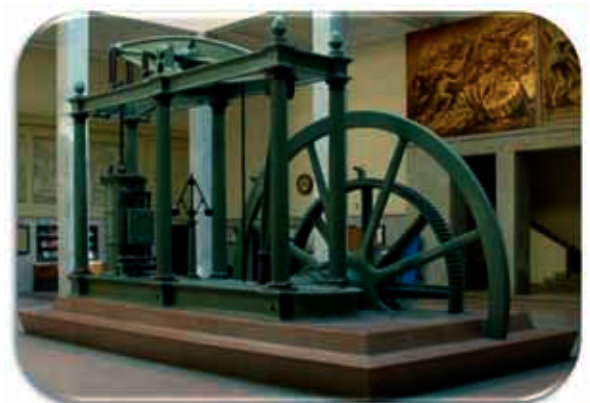
A late version of a Watt double-acting steam engine, in the lobby of the Superior Technical School of Industrial Engineers of the UPM (Madrid).
