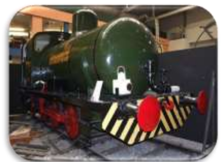
Preserved Andrew Barclay 0-6-0 fireless steam locomotive, South of Scotland Electricity Board, No. 1
