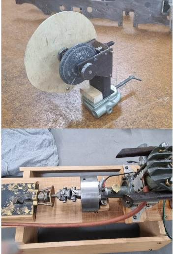
Ron Copeland displayed a two stroke engine with prop shaft. It is water cooled with water forced through the system by the propeller. This was built by the owner's father at the age of eighteen in the 1930's.
