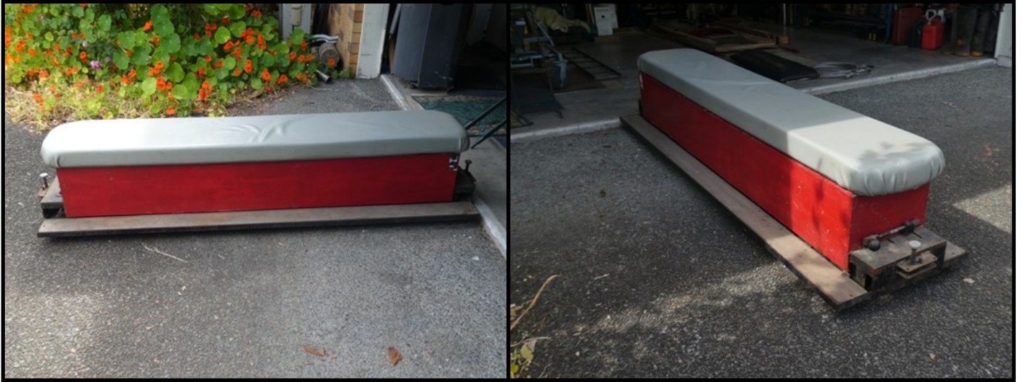
2m long 7 & ¼ Inch Gauge, ground level Trolley Has a hand operated brake on the front bogie
