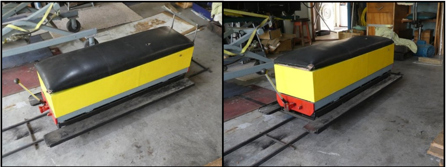
Smaller 7 & ¼ Inch Gauge, ground level Trolley – 1.14m long Has hand operated brake working on both bogies
