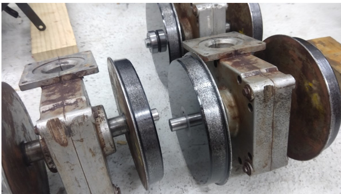
The gouges from contact with the rails on the gearbox cases
