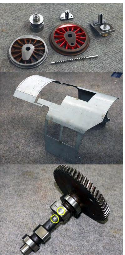
Dave Housley is making more progress on his 0-6-0 version of a Beejax 5" loco, here are two of the wheels the one on the left is to have a tyre shrunk onto it as are the others. The jigs and 3mm broach are so that Dave can cut keyway slots in the wheels before fitting to the axles
