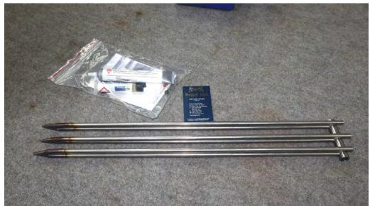
Lastly tonight we had a very nice superheater made by Les Brown, made from stainless tube, tig welded at the hot end. Les is planning on joining to the headers with silver solder paste. The superheaters are for a 5" Rebuilt Royal Scott loco.
