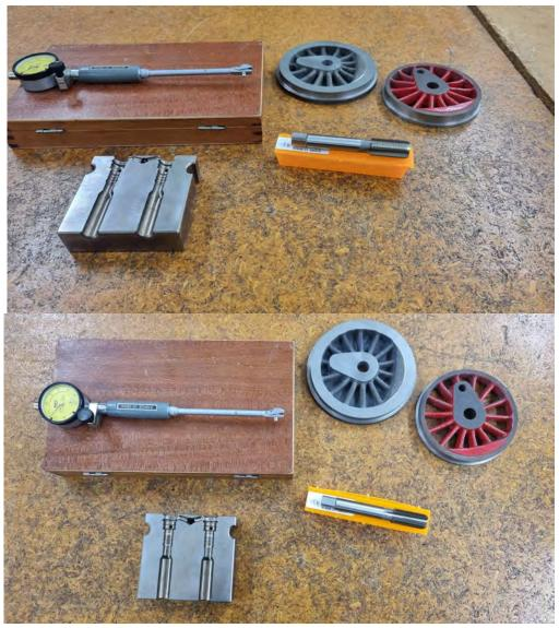
Dave Housley submitted a few items to talk on. The first was a metrology item of a bore gauge which when set with a setting ring or micrometer reads of on the face the size of the bore but remembering that a positive reading is undersize conversely negative oversize. The wheels for his Beejax are turned ready for fitting tyres and the shrink fitting of them was discussed. Also displayed were samples of laser deep engraving (embossed) and details of tap manufacturing.
