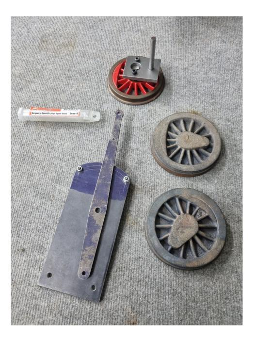
Finally on to Mike Jack who displayed his highly detailed for his BR Class3 tank engine pony truck he displayed the progession of development of patterns of the pony truck frame from actual sand casting through to wax printed patterns. Just to finish off on the table were finished parts for valve gear
