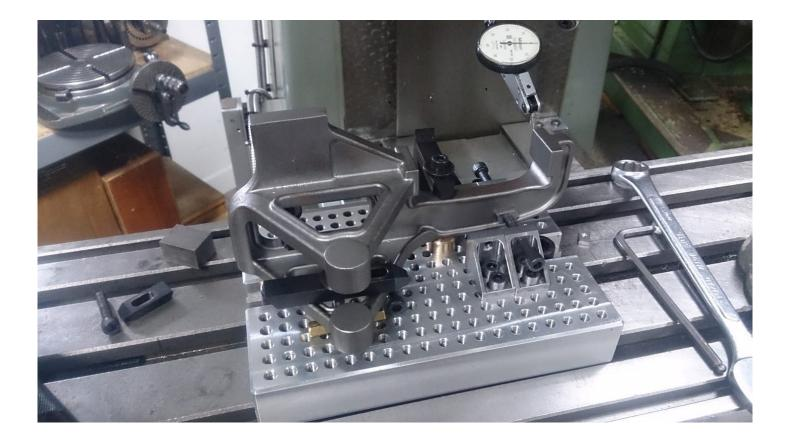
This photograph shows the fixturing plate Mike made for machining this type of casting and some brackets for clamping the part accurately during machining.
