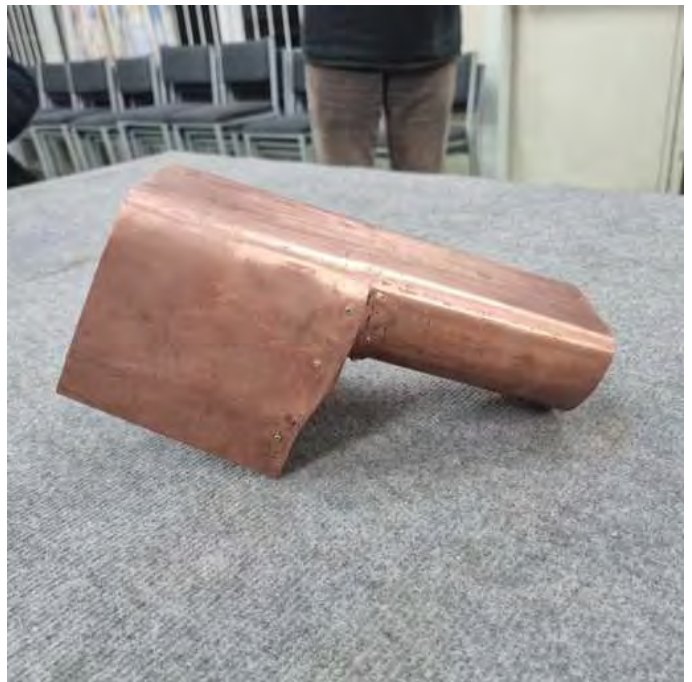
Arnold Van Zon brought in the barrel and wrapper for his 31/2" loco he is building and was asking questions regarding silver soldering techniques and how to not fall into the pitfalls in silver soldering further down the track
