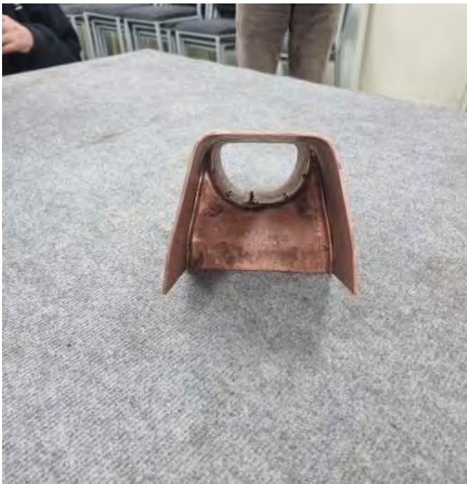
Arnold Van Zon brought in the barrel and wrapper for his 31/2" loco he is building and was asking questions regarding silver soldering techniques and how to not fall into the pitfalls in silver soldering further down the track
