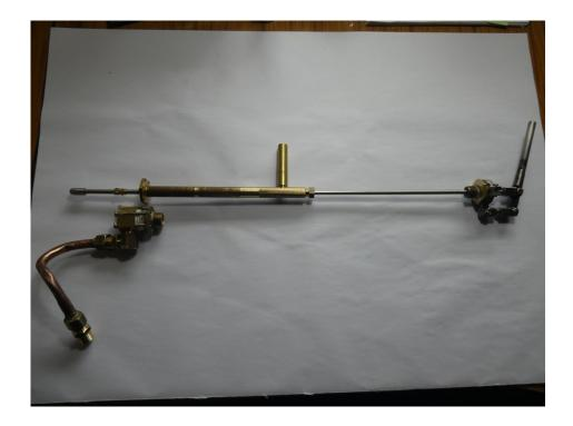
Showing the Regulator fitted plus the two Water Pump By-Pass Valves all plumbed in.
