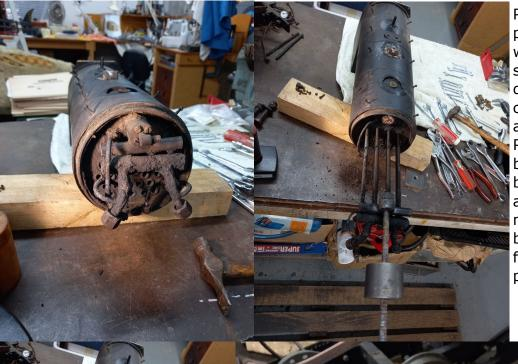
Photo's-8 & 9 With the superheater out I thought I would give them a quick sandblast to see what condition they were in. As you can see I was in full Health and Safety mode with full PPE covering! This work ok but I did use lots of Glass beads to do a small amount of work. I did manage to get hold of a bead blaster I could use for a while for the other parts.
