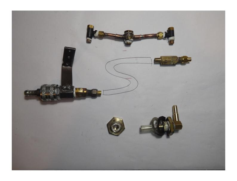
**From Greville**, top item are the two boiler "Top" feed water clacks – one for each axel Pumps as there are two.
