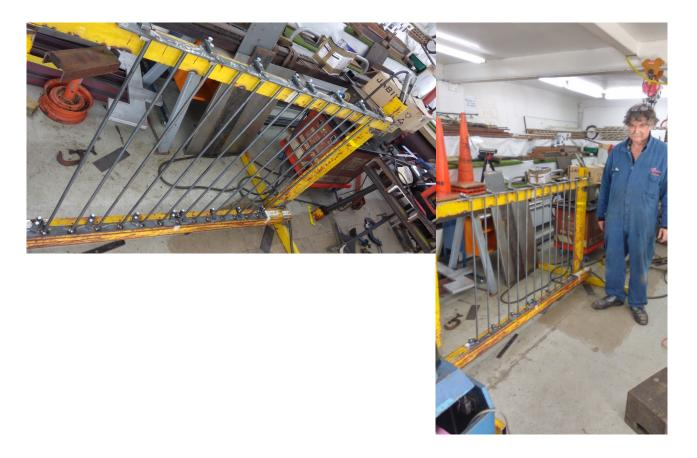
Timothy has completed the jig for the safety fence at the smokebox corner, and welded up the first two panels with material that Allan Bailey and Grant had prepared over the last few Saturday working bees. When the posts for these panels are completed, they will have a trial fitting, and then be sent to the galvaniser. Eventually another 20 similar panels will need to be manufactured.
