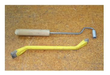
From the floor we had some what are they items, the top one is a roller used when laying up fibreglass and used to squish and roll the resin into the matting. The lower yellow one was a double ended abrasive touch up stone for commutators.
