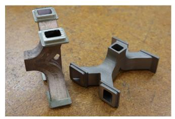
These manifolds are for Mike Jacks class 3 project locomotive. The one on the left was from an original batch of castings that needed to be modified to fit inside the large and complex smoke box saddle fabrication. The right hand one was made via investment casting and should have worked out a bit cheaper but due to a miscommunication at the foundry the price was quite a bit more than expected.
