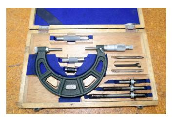
Peter Woodford brought in a NSK made in Japan 1 - 4 inch Micrometer, yes in imperial. The mic had a bit of rusting but came in its wooden box with test pieces and extension anvils. Quite a nice tool.
