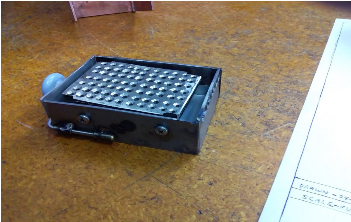
The Rosebud grate being built by Greville for his new Beejax
