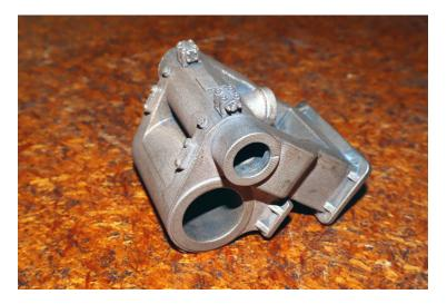
Mike's last offering tonight was an outstanding small cylinder casting for a Gauge 1, 4-8-2+2-8-4 Garret locomotive model of a Rhodesian Railways engine. The casting was cast from wax patterns in silicon bronze.
