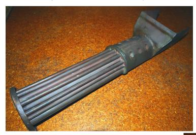
A new visitor and prospective future member **Ar-nold van Zon** brought along a partly built boiler for a 3-1/2" Highland Lassie. This is the same type locomotive that Bruce Cooper is currently rebuilding, Unfortunately the boiler had a few issues that would cause it to fail our boiler code. Some of the tubes were so close together as to be touching and the combustion chamber had a straight join that had been brazed.
