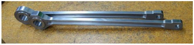
The two large connecting rods are for a customer in the USA who is building a 7-1/2" gauge 2-8-2 USA Mikado. Michael has machined these from a piece of black mild steel bar and has spent a lot of time in the finishing of them with his polishing stones of different grades to get a very nice grain and smooth finish to them.
