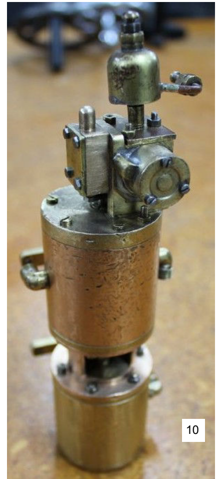
Photo-10 Bruce Cooper has one of his locos in bits and is doing his usual nice job of rebuilding it back to as good as new condition. He had with him the steam water pump off it and was wanting to know more about this pump and a little bit of how it works with regards to the steam valves and the little shuttle valve it has. By the looks of all the little dents on it someone thought the only way to get it to go was to tap it with a spanner (many times). This is an old railway trick that usually causes more damage than any good. When he pulled it apart he found out why it wouldn't go. The water pump aluminium piston had just about corroded away from sitting around for so long with water still in it; other parts were seized as well.
