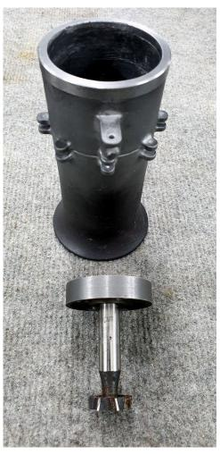
Mike had a number of new castings to show us now that the lockdown is over and the foundry is open again. Included were a cylinder that had blocked steam ports and took forever to clean out. More successful were the petticoat pipe and chimney stack, all for 7-1/4" gauge engines. And finally some brake blocks for his Class 3 project.
