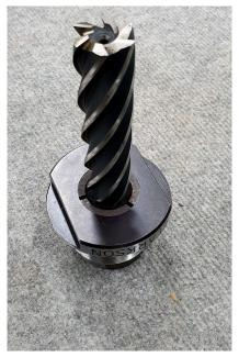
Mike Jack is restoring an old shaper that he has. Part of the job required the use of this large end mill cutter. Mike noticed that it would not run true and after much head scratching and pondering he discovered that the Clarkson chuck he was using had been ground incorrectly during manufacture, and this caused the cutter to wobble.
