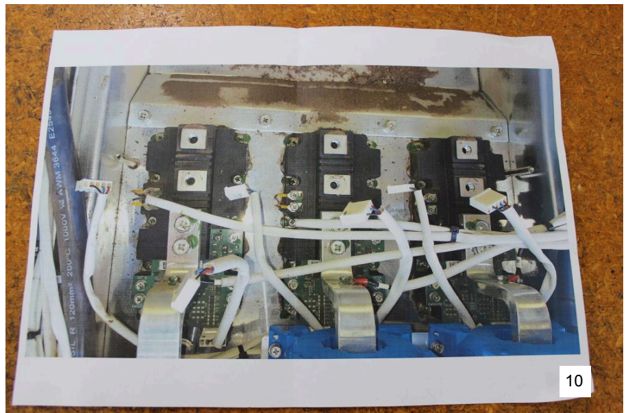
Photos-9 & 10 also from Tim are parts of an IGBT 1/2 bridge, An H-bridge is an electronic circuit that switches the polarity of a voltage applied to a load. These circuits are often used in robotics and other applications to allow DC motors to run forwards or backwards. In this case this motor is off an old Planner type machine. In the first photo you will see the one that has let the smoke out, and it's no good anymore. The second photo is what it should look like in operation.
