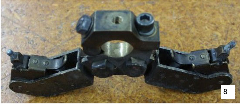
Photos-7 & 8. Timothy Robinson has been working on the overhaul of some big electric motors for a customer. Upon stripping the motor down it was found that it had problems with a couple of the brush holders and with the age of the motor it was not easy to find a direct replacement for them so he has had to make something that is very close to the original one to fit the motor.
