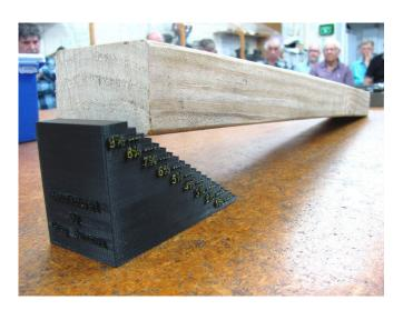
**Greg Burrows** 3D printed up this gradient gauge. When used with the correct length piece of timber he will be able to dig the correct gradients for his garden railway.
