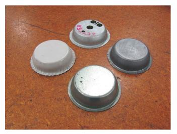
These sample pressed cups where brought in by **Peter Woodford** to show the different quality of finish that can be produced when using press tools on sheet metal.
