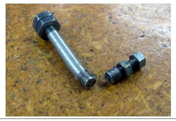
This damaged - and another broken - spring pins are from Grant Anderson's Beejax loco variant.
