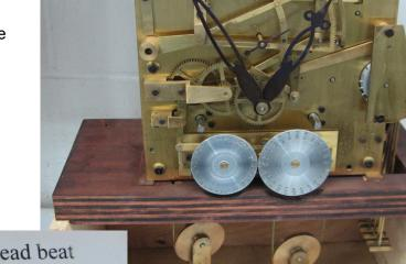
Long case clock movement with dead beat escapement and differential drive for the chime and strike.
