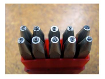
**Mike Banks** brought in a set of reverse number punches obtained at a club auction. These could be punched into a mould to produce a raised character in the finished work or punched into thin sheet metal to produce a raised imprint on the reverse side.
