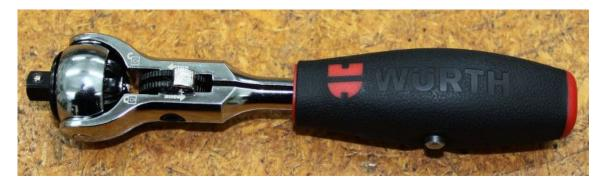
From **Greg Burrows** is a nice little <sup>1</sup>/<sub>4</sub>" drive for a socket set that he bought from one of the tool companies that call into work. It is a very flexible unit with the head being able to swing through 180 degrees from one side to the other. (This is how you get the ratchet to work in both directions). The handle also will open up to form a Tee handle that is useful for tapping-type operations.
