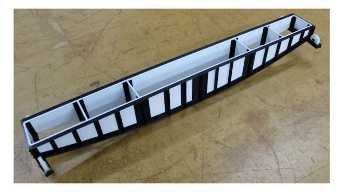
Also from Greg Burrows is the start of the turntable for his NZR garden railway in 1/24<sup>th</sup> scale. The turntable is made up of ABS white plastic sheet 3mm thick and the black parts have been 3D printed in ABS with all the rivet detail printed into them and all glued together with MEK. A couple of meetings ago he brought along the little motor and gearbox that will be used to power it around.
