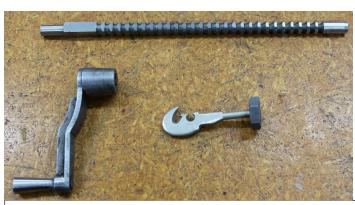
thread from the as-cast condition. It worked well but he was very disappointed with the quality of the die nut as it does not run true with the thread. And we can confirm that Michael's thread is running true with the rest of the job. This photo shows how much the die nut runs out.
