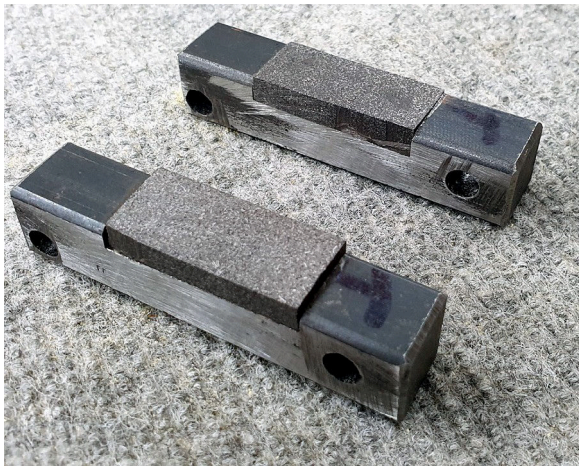
Greville Wills has made these brake blocks for a ride trolley using discarded disc brake material cut and glued into the steel brake blocks.
