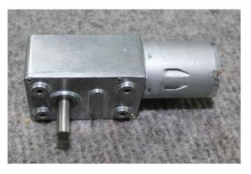
Also from Greg Burrows is a nice little stepdown motor and gearbox to be fitted to the 1/24<sup>th</sup> scale turntable he is building for his garden railway. The motor is 12 volts and the gear reduction is down to 10RPM on the output. These came from China from Banggood at a very reasonable cost.
