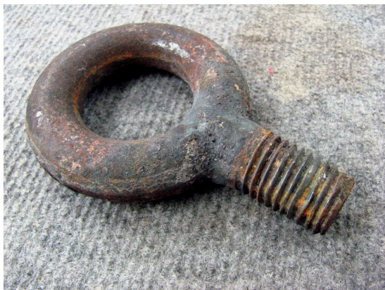
Tim Robinson had to repair the thread in an electric motor where this eye bolt had stripped the thread out on removal.
