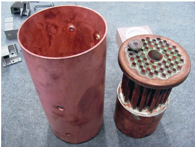
A stationary test boiler is being finished by visitor Bill Parker after the owner came to Bill for help. Bill says a handy tip is to paint with "Twink" where you want to mask to prevent silver solder getting where it's not wanted.
