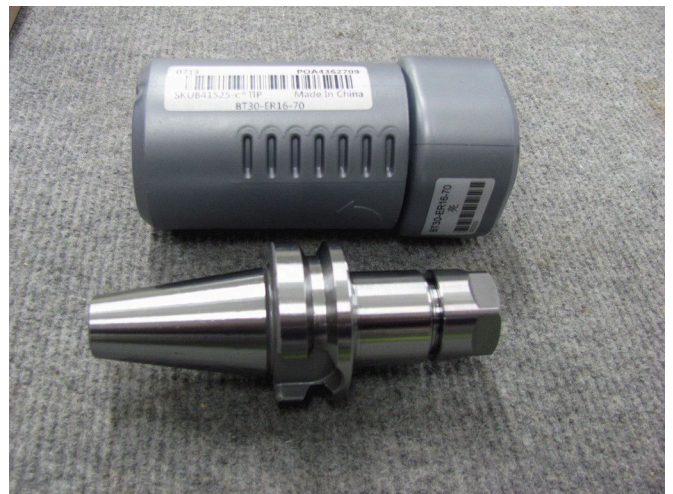
Pete Woodford has landed another collet adapter from China, this one is BT30 to ER16. Pete says this one is good and true.
