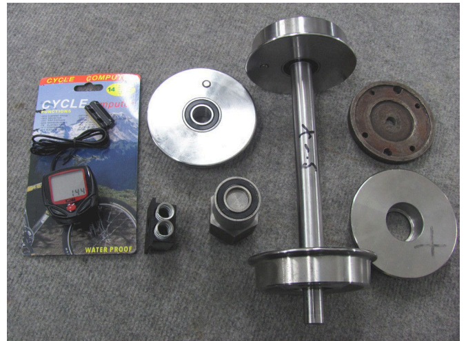
Part of the same job is the assembly of the bogies being undertaken by Grant Anderson . Grant has made a couple of dollies so that the bearings can be pressed into the wheels squarely. You can also see where a magnet has been put on the inside of a wheel to operate a speedo on the trolley.
