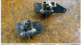
These little bronze castings were made by **Mike Jack** for a client, they are dummy rocking grate mechanisms for a 9F Britannia in 5" gauge.
