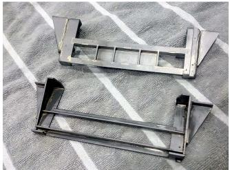
Mike has also put together from laser cut parts these rear side tank frames for his 5" gauge 3MT locomotive project. The next picture shows the mounting box for the cab reverser gear, and Mike has made a bronze tubular casting that is easy-flowed into it so that the side tank water balance pipe (the U shaped hollow bronze castings) can attach to the box and allow water to flow through without causing any corrosion. Once again all very professional work turned out by Mike.
