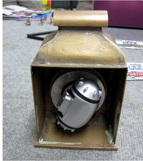
This headlight by visitor Bill Parker is being built using a Head Light LED torch as the source of light. This looks like it will do the job and fits inside the unit perfectly.
