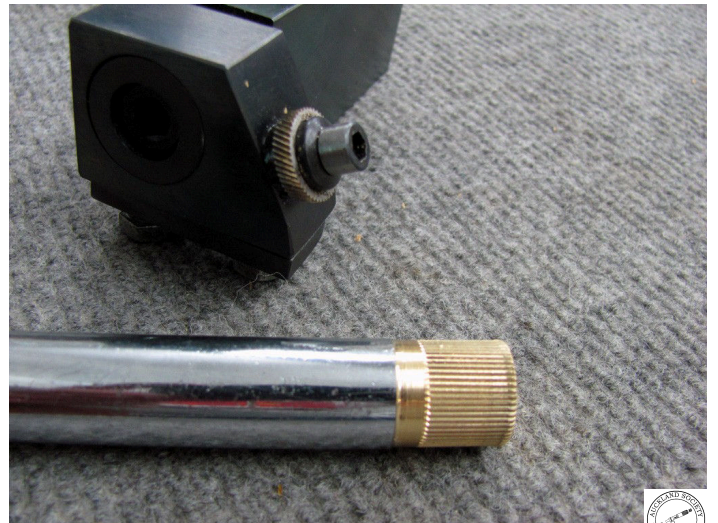
Sorry not quite sure who it was who made this straight knurling tool and sample piece, but it was a nice job and looked like it worked well.
