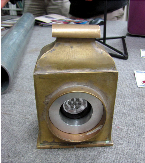
This headlight by visitor Bill Parker is being built using a Head Light LED torch as the source of light. This looks like it will do the job and fits inside the unit perfectly.
