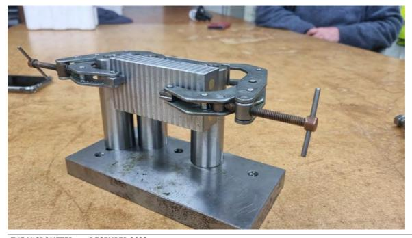
Mike Jack had a first principle exercise whereby a plate ground parallel is tapped and rollers are turned ,drilled clearance for caphead screws then ground exactly parallel between centres and the ends ground on the same centres which creates a square face .Then havingdrilled and tapped the plate the rollers can be fixed in the upright attitude and will naturally be square to the plate
