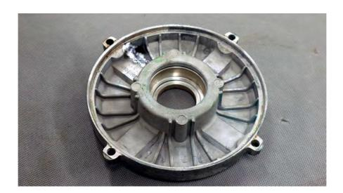
The end plate from this electric motor is from a motor that Mike Moore wants to use on his lathe, the only problem was the plate was cracked to the extent it was not useable, as a replacement was not easily obtainable Mike has had the part welded and it should do the job nicely.
