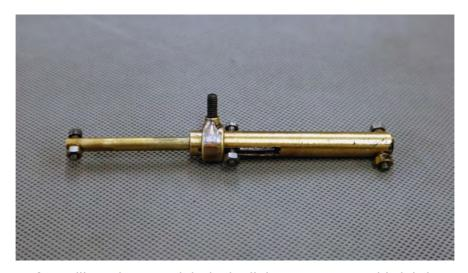
The last item of Greville's pieces tonight is the linkage to connect his lubricator to the motion of the locomotive, by limiting the movement of the sliding piece will control the stroke of the arm on the lubricator easily providing control over the oil flow to the cylinders.
